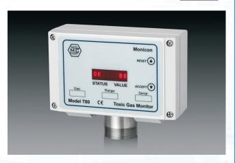
The T80-CO is a 4-20mA, 3-wire transmitter. It is housed in a rugged, compact metallic enclosure. It incorporates advanced SMT electronics and an amperometric electrochemical sensor based on micro fuel cell technology, designed to be maintenance free and inherently stable.
