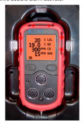
Fig. 4-10 Instrument in Alarm Condition
