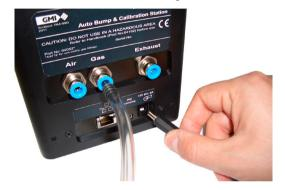
Fig. 2-8 Connect Power Supply to Station
