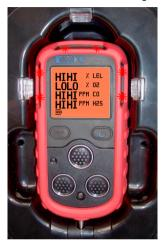
Fig. 4-11 Instrument in Alarm Condition
