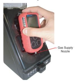
Fig. 4-15 Lift Instrument Clear of Gas Nozzle
