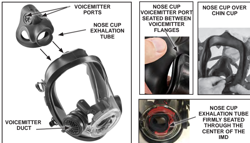
FIGURE 19 INSTALLING THE NOSE CUP
