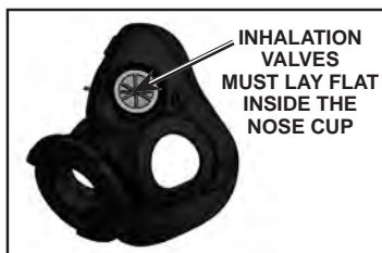
FIGURE 1 CHECK INHALATION VALVES ON THE STANDARD NOSE CUP
