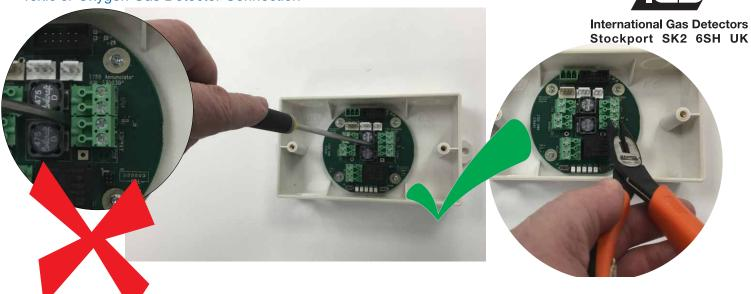
When unplugging detectors from the main PCB DO NOT lever them off. This will potentially cause damage to the PCB and/or connector mating parts and invalidate any warranty. If it is necessary to remove the PCB connectors use long nose pliers.
