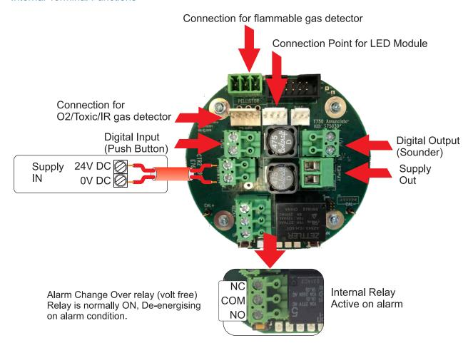
NOTE: The unit is shipped configured and Pre-Calibrated for its detector and options and alarm levels
